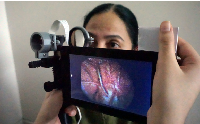
A prototype of a tablet-based multispectral retinal imager.
