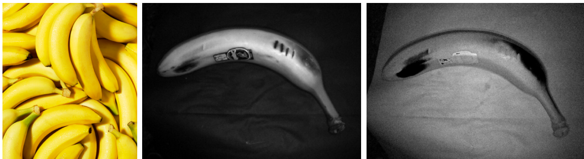
Multispectral measurement of internal and external bruises in bananas in two different IR channels images external bruises, including four superficial notches on the banana skin (center), and internal bruises (right) on a banana. As the right-hand image shows, the banana meat is decayed at the bottom and the top. Left: Getty Images
