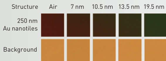
Experiment showing the different color changes when different thicknesses of SiO 2 were deposited on the chip.
