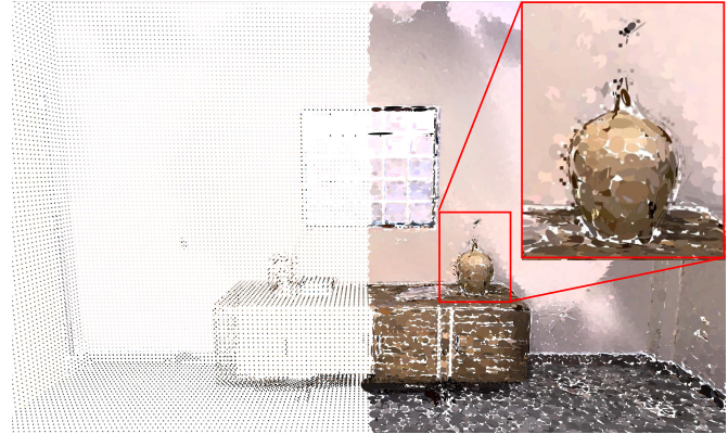
Fig. 1: Demonstration of voxelized surfels. VSS-SLAM divides the underlying scene using voxels (left) and then generates surfel representations of the scene (right) based on the information within the voxel vertices.
